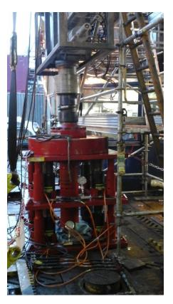
stroke and pulling force can be achieved by stacking tension tables and adding hydraulic cylinders.
